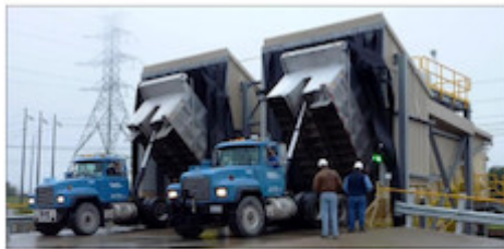
Fig. 1. Example for two truck Reception Samson® Material Feeder from AUMUND (showing a similar situation as National Gypsum Shippingport, photo AUMUND)
