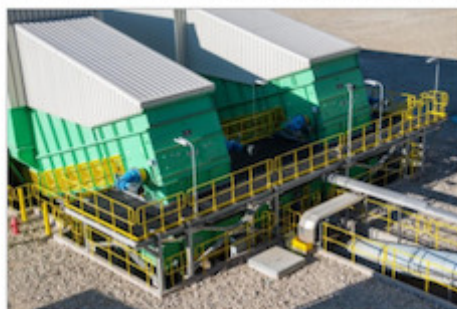
Fig. 2. Example for two Storage Samson® Material Feeder from AUMUND (showing a similar situation as National Gypsum Apollo, photo AUMUND)
